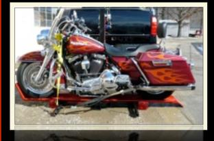
We recommend that this hauler be used by vehicles with a class IV or V hitch. The heavier the hitch the better. The receiver size needs to be 2" square or else you need a receiver reducer. Please consult with your vehicle or hitch manufacturer for complete requirements and specifications for your specific hitch.
